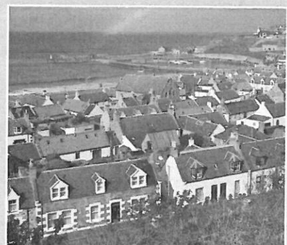
Cullen Seatown, Moray. In this conservation area the layout of the buildings is closely linked to the landscape context: on the north side of the village gables face the sea to maximise shelter; here on the south side the houses are aligned to maximise light. © N. Haynes
